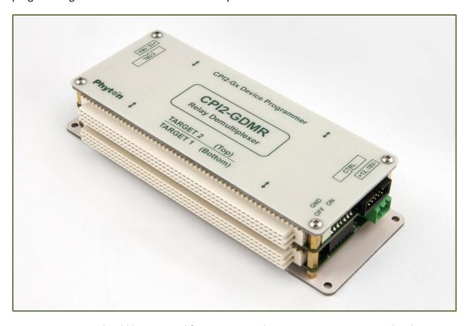
A CPI2-GDMR unit should be powered from an external 12 to 18V@2A power supply. The unit has a couple of two-pin green power connectors to plug a cable or wires from the power adapter, which can be connected to either side, wherever it is more convenient. These connectors are located on both short end faces of the CPI2-GDMR unit. See the CPI2-GDMR side view below.
